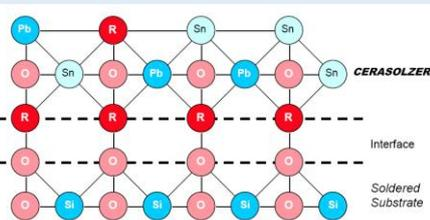
When quartz glass is soldered, the metallic oxides (R/O, which are components of Cerasolzer) unite chemically with the SiO<sub>2</sub> of the glass.
